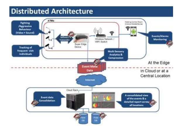
In a distributed design, the Smart Compression can be deployed on a Super Edge device close to the camera resulting in a saving of both storage and network bandwidth.
